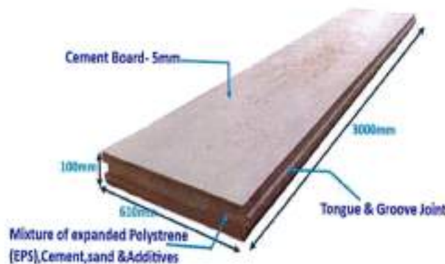
NON-LOAD BEARING ECO WALL PANELS ASSEMBLY - 100mm THICK
