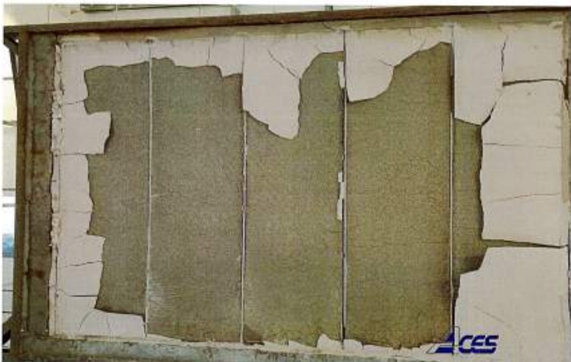
The unexposed face of the specimen after the test
