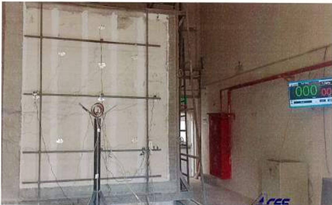
The unexposed face of the specimen at commencement of the test
